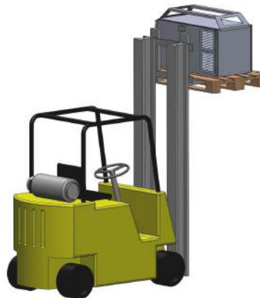
Fig. 4.3.3 Transport and mounting of the ITW GSE 2400 Compact by means of a fork-lift truck
