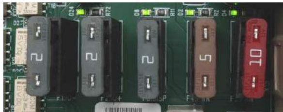
Fig. 9.0.1 Fuses F1-F5 and LED indication (A2 Interface Board)
