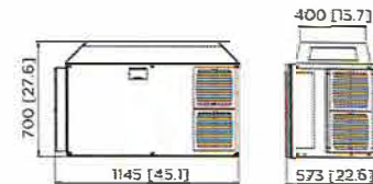
Converter for under-bridge mounting
